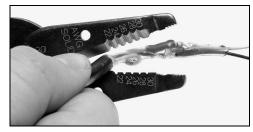
For Wiring Diagram B installations, remove the Uniden adapter segment at the end of your data cable as shown at left. Snip off the end of the cable protected by the black heat-shrink. At right, we have used clear heat-shrink for clarity, so you can see the diode and resistor protected within. Remove this portion of the cable.
